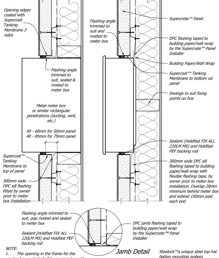
1. The opening in the frame for the meter box or duct shall be prepared exactly as for windows and doors, refer to Detail No SPC 4-3, page 43
